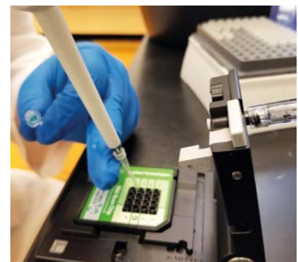
Philip loading RNA Nano Chips to determine the quality of RNA from injured tissue samples.
