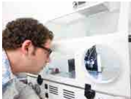
Ed uses the ultrasonic atomisation machine to coat sheets of polymer with tacrolimus
