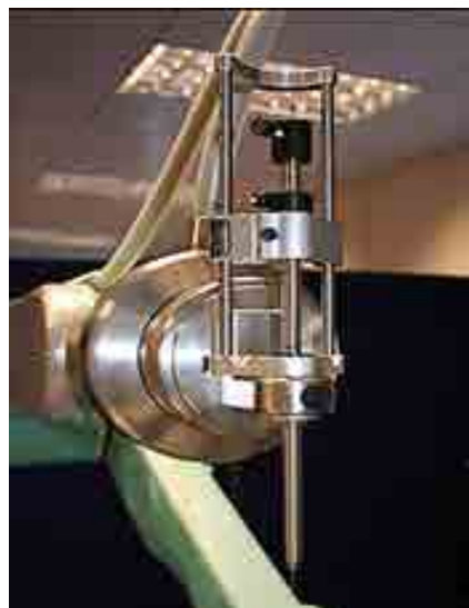
A neurosurgical robot is used to increase the accuracy and safety of implanting catheters in the brain
