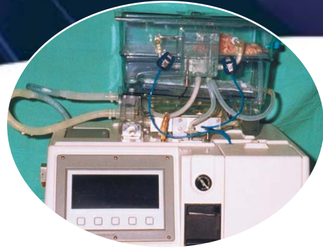
The Waters RM3 machine used for pulsatile pancreas perfusion in this study.
