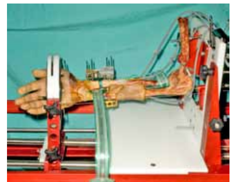
A cadaveric specimen under investigation using a custom-built biomechanical jig. Green joint pressure sensors can be seen mounted within the joints. External fixators can also be seen affixed about a simulated distal radius fracture. Note that the clamp holding the hand is pneumatic and can be easily rotated through the arc of forearm rotation to replicate normal forearm movements. A 5kg weight loads the forearm across the wrist via a series of cables and pulleys.
