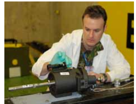
John adjusting the gas gun used to fire fragments at novel body armour materials and designs.
