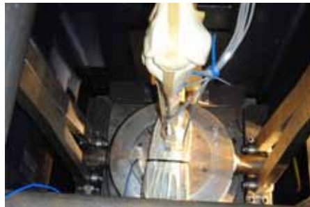
The synthetic foot model sits on the 45kg plate, which is capable of accelerating to 45mph within 10cm.
