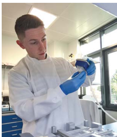
Conor using the PyroMark® Q24 Vacuum Workstation to bind amplified DNA to streptavidin beads.
