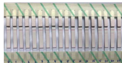
Lateral flow immunoassay at work showing varying concentrations of PSA solutions (0-25ng/mL; numbered in blue below each strip) – note the gradient in colour intensity of the test lines with varying PSA concentrations.
