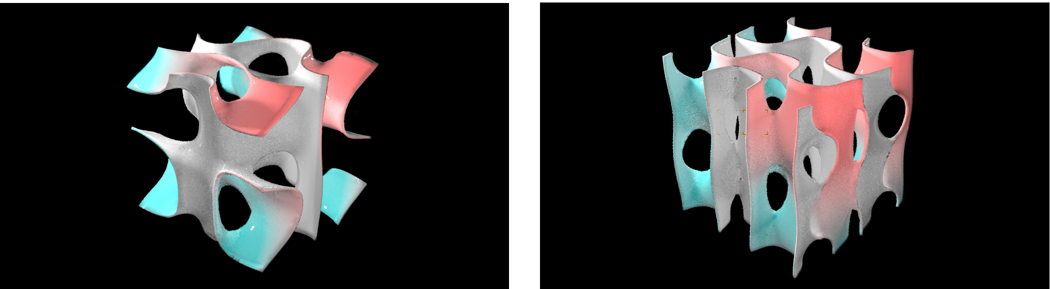
Fig 1. Variation in co-efficients A, B, C in the equation: A*\sin x \cos y + B*\sin y \cos z + C*\sin z \cos x = 0 This creates lattices with different anisotropy and density.
