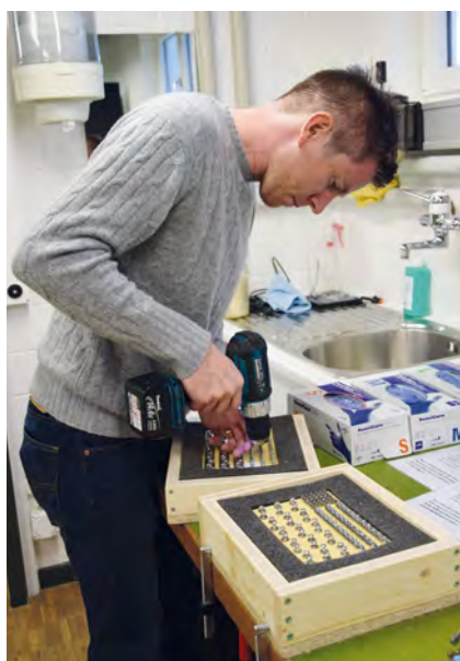
Preparing jigs for testing screw tightness.
