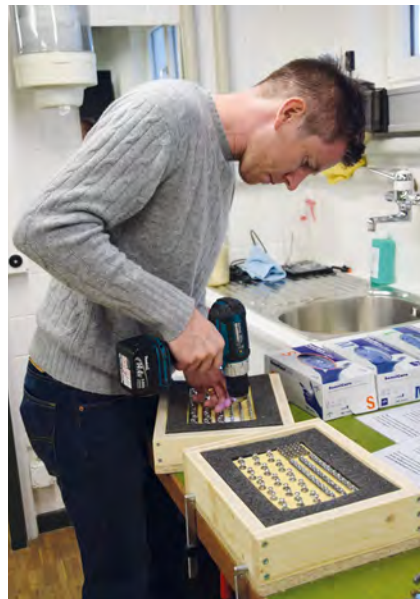
Preparing jigs for testing screw tightness.
